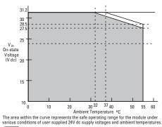
= Normal mounting safe operating range, (includes \_\_\_\_\_\_).
