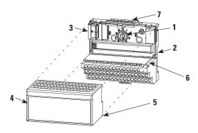
The module mounts on a 1794 terminal base.
