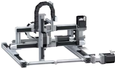
Lexium MAX Multi-axis systems for 2 or 3-dimensional positioning solutions
