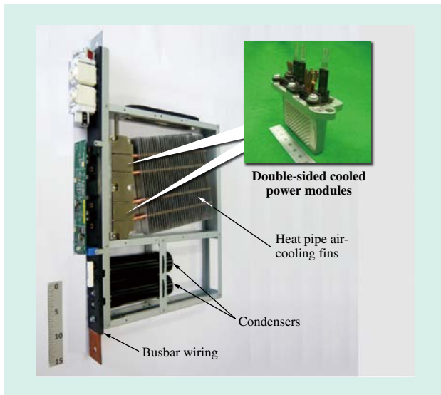
Fig. 6—Modular Power Conversion Unit. Two power modules and condensers are placed in a straight line, enabling a lighter weight and thinner design with a width of 5 cm.
