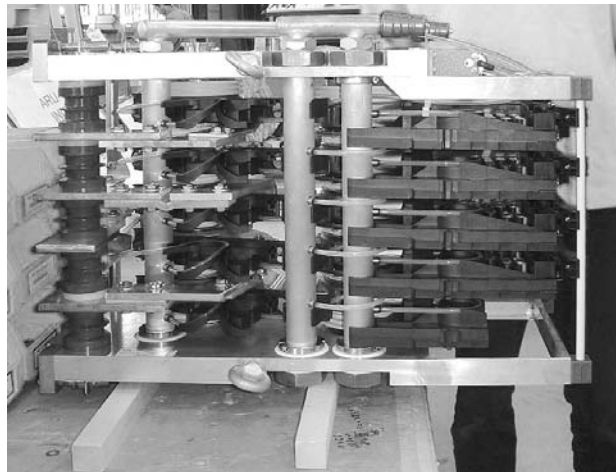
Figure 6-2 Phase Module Placed on two Wooden Beams
