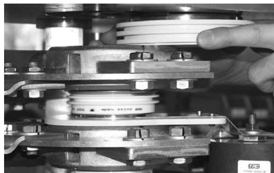
Figure 6-4 Removing Isolator Disk
