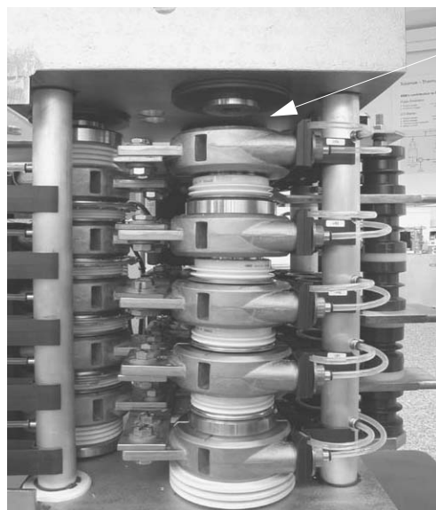
Figure 8-19 Removing Top Isolator Disk
