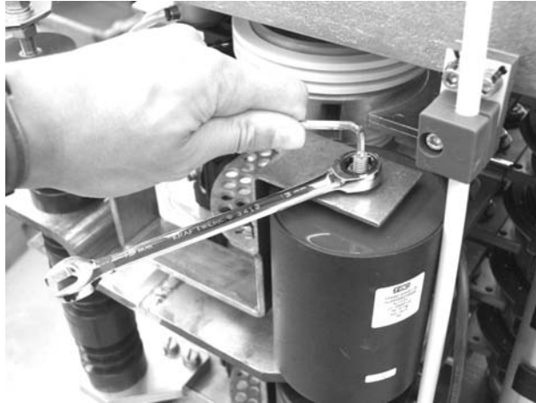
Figure 8-6 Removing the Top Fastening Nut
