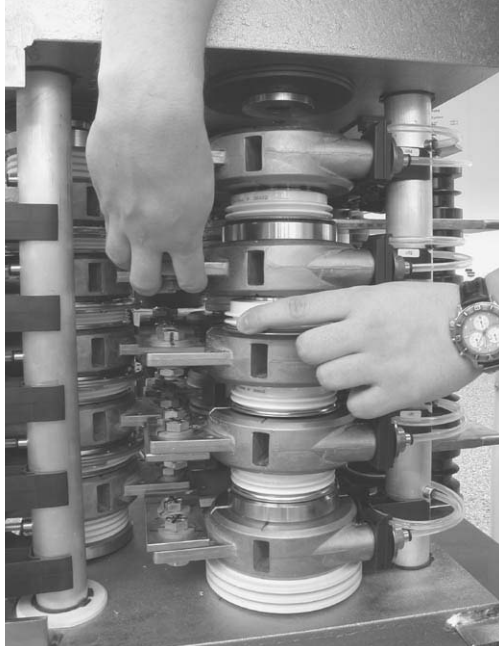
Figure 8-20 Removing the Diode
