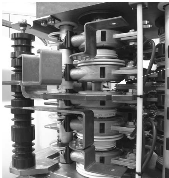
Figure 8-16 Upper NP Diodes Removed
