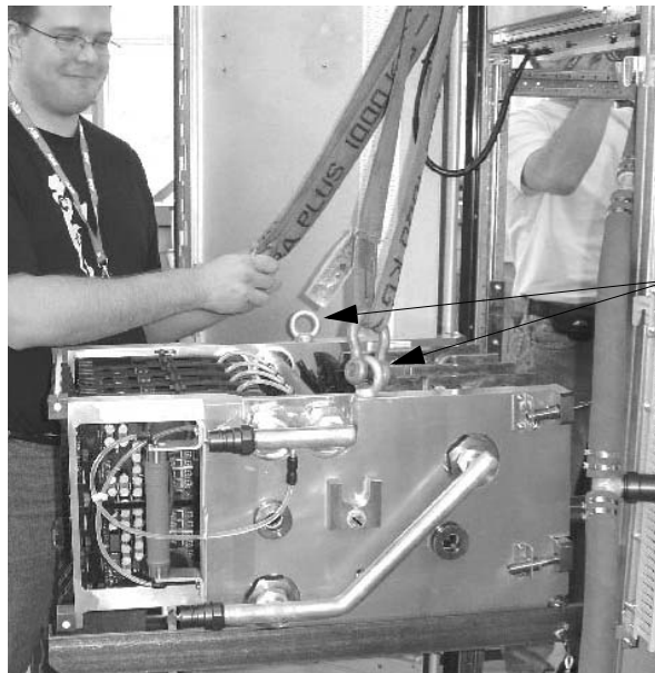
Figure 4-11 Phase Module Attached to Crane
