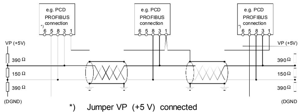
The PCD7.T160 termination boxes should be used to terminate the bus cleanly :
