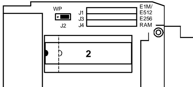
Insertion of jumpers allows the following memory chips to be fitted :
