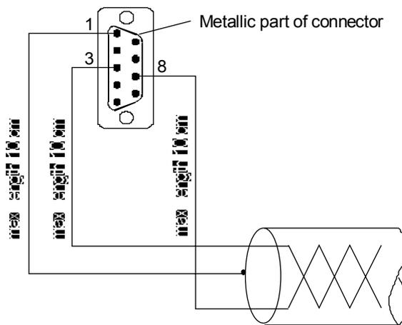
The unshielded part of the cable at any connector, and from the shield alone to pin 1, should not exceed 10 cm.
