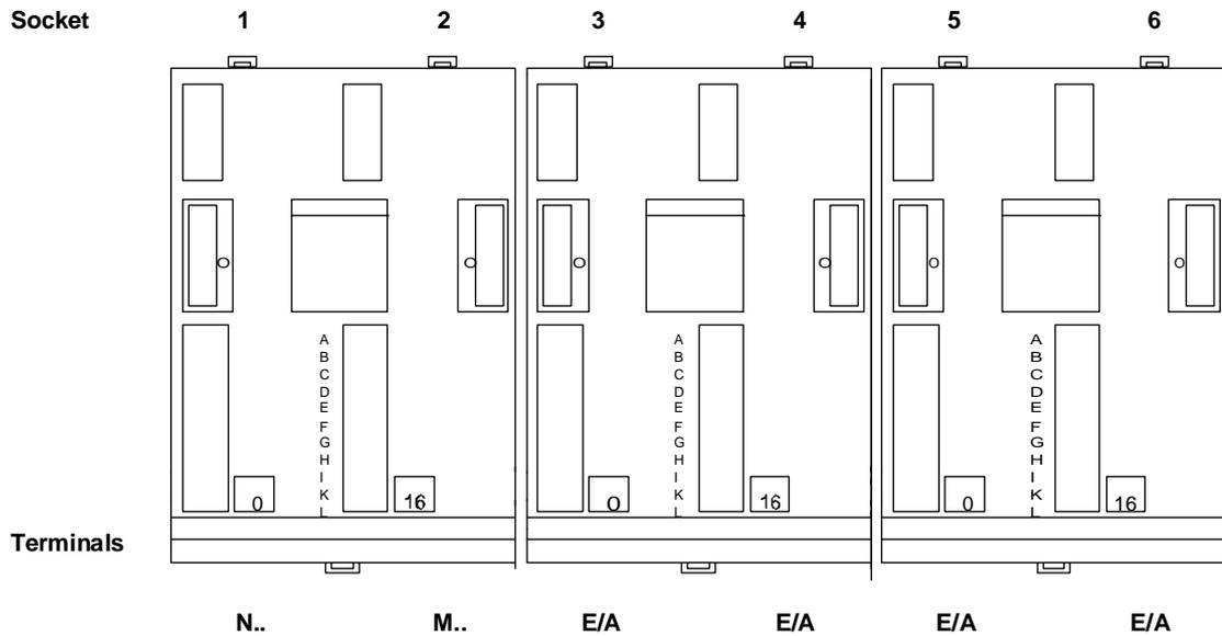
Socket no. 1 for power supply module PCD4.N2..
