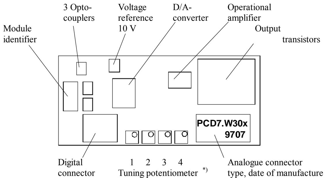
\*) These potentiometers are factory set and **should not be** adjusted by the user.
