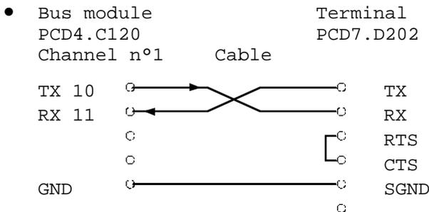
15) Make up the cable for connecting the PCD4 and the terminal in MC0 mode (no control lines needed).
