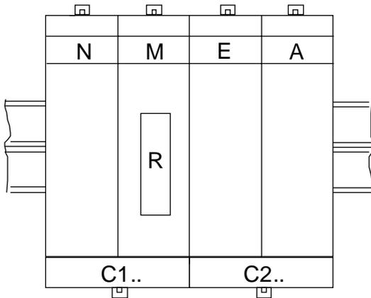
14) The following modules must be present for channel 1 to be used as an RS 232 interface :
