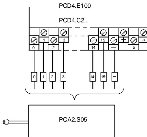
6) The PCA2.S05 applies +24 VDC to inputs 0 to 15 via the switches. This can also be obtained from an external power source.
