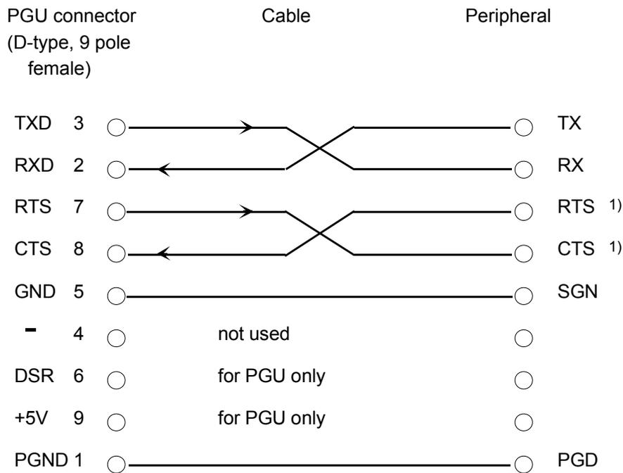
1) When communicating with terminals it is necessary to check whether certain pins should be provided with bridges, or whether they should be set H or L with the SOCL instruction.
