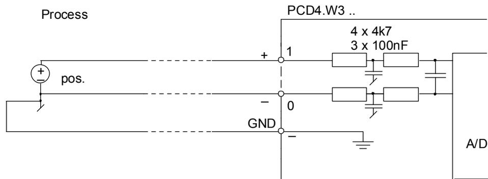
**Note :** The process ground, or that of an input amplifier, must be connected to the ground of the analogue module (at terminal " - "). Instead of a separate ground line the shield of the cable can be used.
