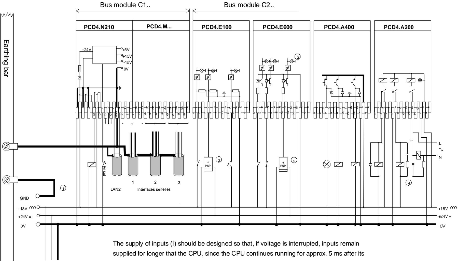
The supply of inputs (I) should be designed so that, if voltage is interrupted, inputs remain supplied for longer than the CPU, since the CPU continues running for approx. 5 ms after its supply has been cut.
