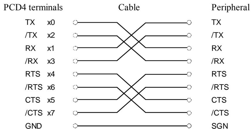
Adapt connector type and connections according to the peripheral.
