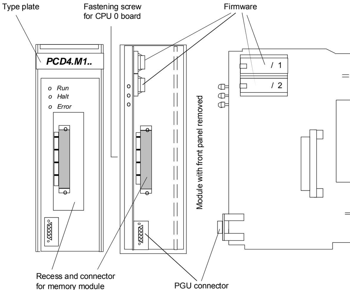
To update the firmware, remove the processor module (cartridge) from the bus module, then remove the front panel from the processor module and unscrew and take out the board. Now both EPROMs can be easily changed. Re-assembly is done in the reverse order.
