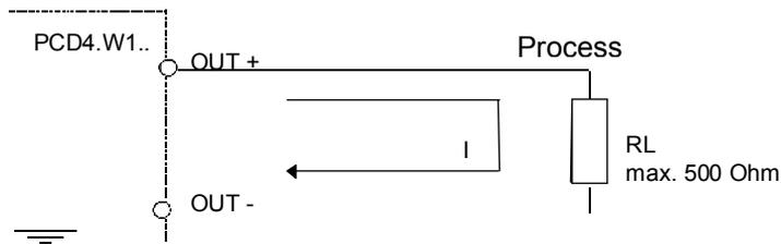
For supplying current outputs, the " + " terminal must be connected to +24 VDC. This supply can be that same as that of the power supply module PCD4.N2.. with a maximum current requirement of 60 mA.
