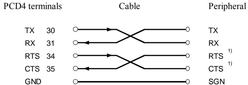
Adapt connector type and connections according to the peripheral.
