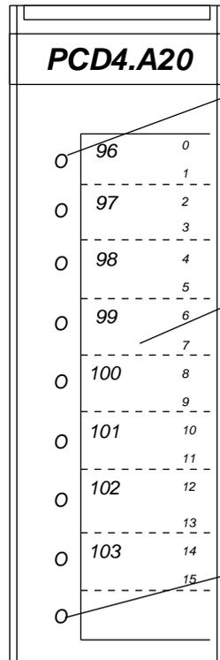
LED display indicating the signal states of the outputs (independent of external module supply).
