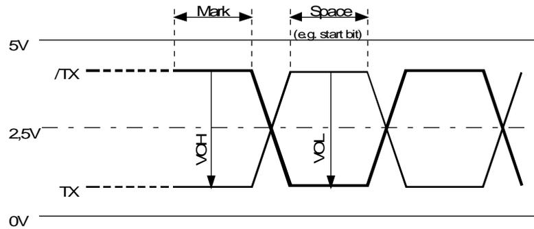
VOH = 2 V min (with load) to 5 V max (without load)
