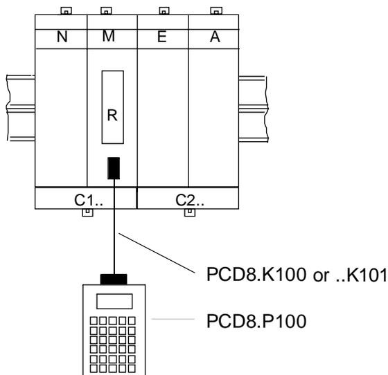
7) Use cable PCD8.K101 to connect the PCD8.P100 programming unit to the PGU interface. (or the former ..K100 cable).
