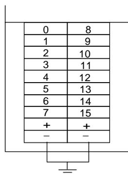
The terminals are always numbered from 0 ... 15. The absolute output address is determined by adding the basic address of the module to the terminal number.
