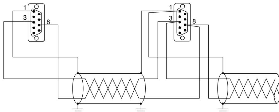
Care should be taken to ensure that the bus line still remains continuously connected when one or more plugs are removed.
