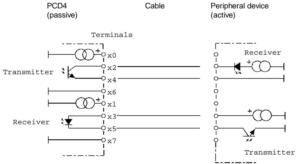
**c) PCD4 transmitter and peripheral transmitter active**
