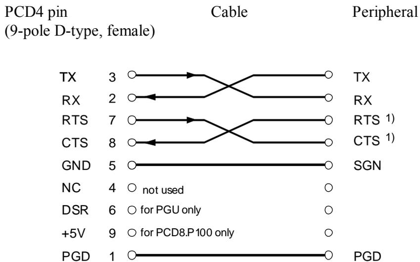
Adapt connector type and connections according to the peripheral.
