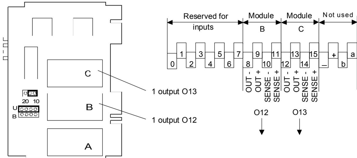
**Installing at space B and/or C**
