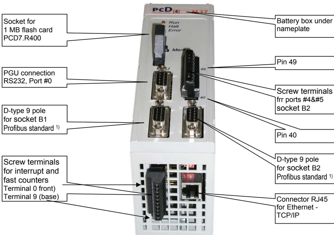
1) The pin configuration of these two D-Sub connectors (9 pole female) complies with the PROFIBUS standard. The two D-type connectors should preferably be used for PROFIBUS networks. Further serial ports should, if possible, be connected to the 10-pole plug in screw terminals.
