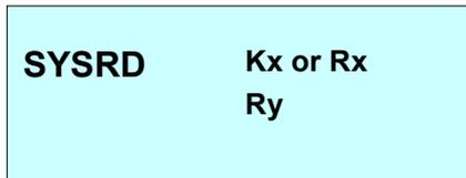
Where: **Kx** or **Rx** is the constant or register with the function code.
