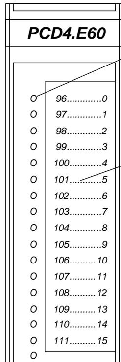
LED display indicating the signal states of the inputs.
