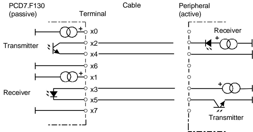
**c) PCD4 transmitter and peripheral transmitter active**
