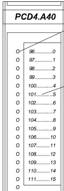
LED display indicating the signal states of the outputs (independent of Ua).
