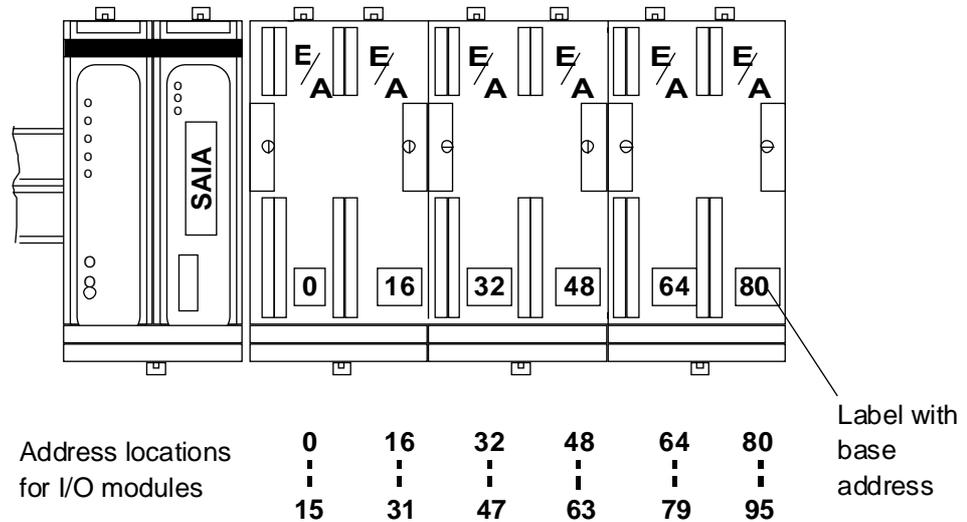
Each add-on I/O module reserves 16 addresses. Starting with the base address 0 (zero) at the first module position to the right of the processor module, the addresses increase towards the right in steps of 16. The same also applies for modules which occupy only 8 addresses. If modules with 8 addresses are used, 8 addresses are lost for each module.
