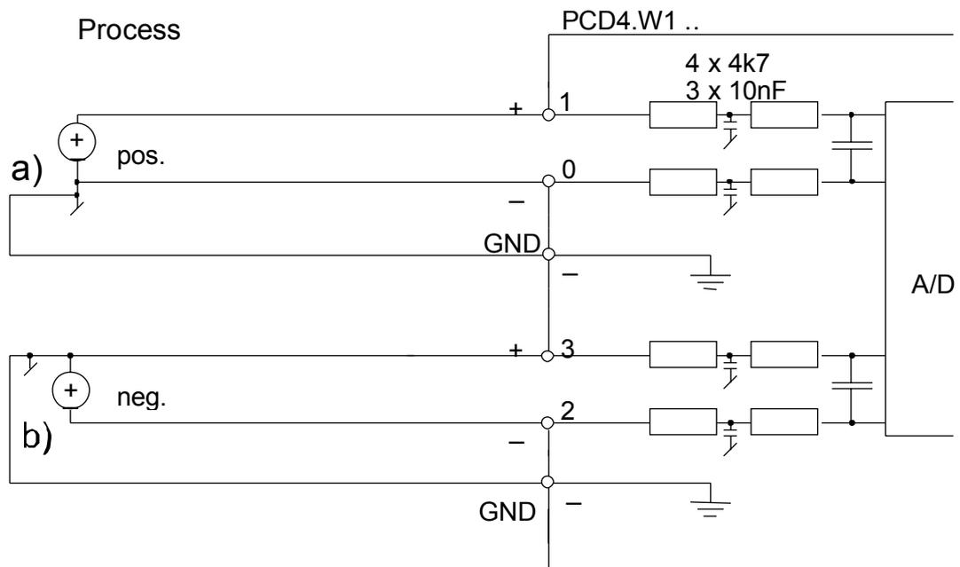
**Note :** The process ground, or that of an input amplifier, must be connected to the ground of the analogue module (at terminal " - "). In unipolar operation, the more positive potential is connected to the " + " terminal. In this way, negative voltages (b) can also be measured.
