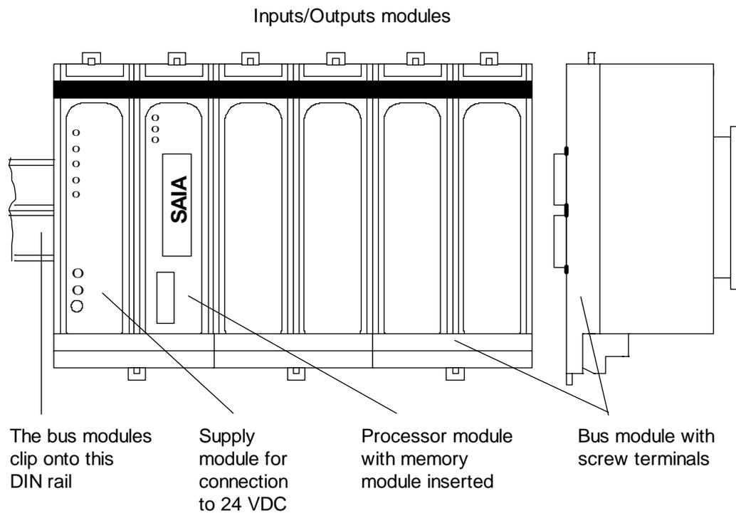
A double mounting rail (35 mm, DIN/EN 50022) is used to support the bus modules. The required number of bus modules are snapped onto this rail and connected together electrically and mechanically (see drawing on next page). External connections should be wired next, using the screw terminals.
