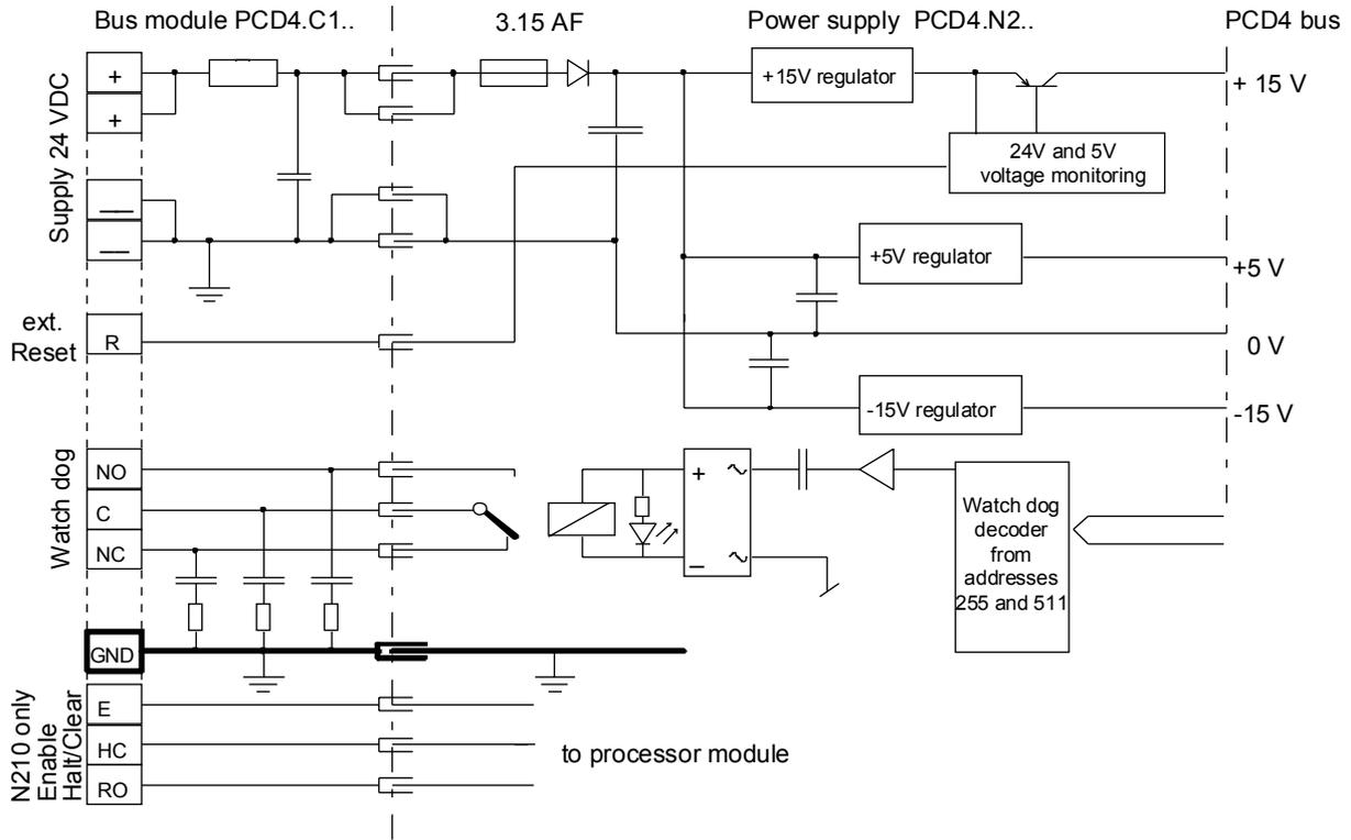
**Screw terminal connections of PCD4.C1x0 or ..C340 bus module**
