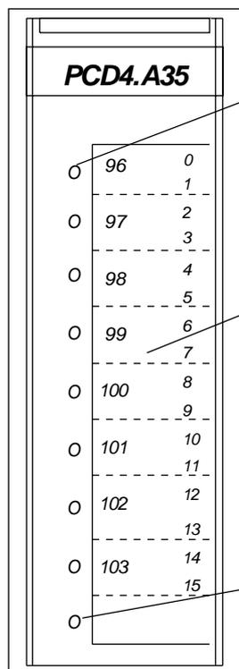
LED display indicating the signal states of the outputs (independent of external module supply).
