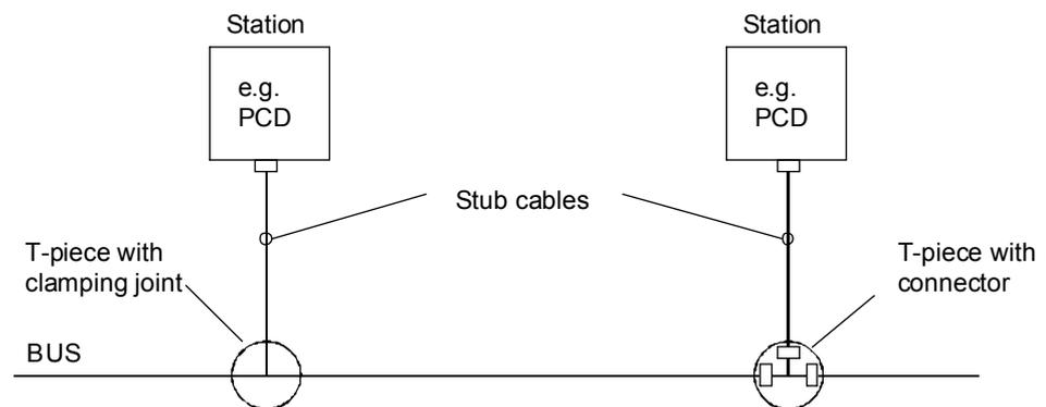
In the case of a wiring plan using stub cables, care should be taken to ensure that the shielded stub cables are no longer than 100 cm for a transmission speed up to 19.2 kBit/s, and no longer than 30 cm for 500 kBit/s.
