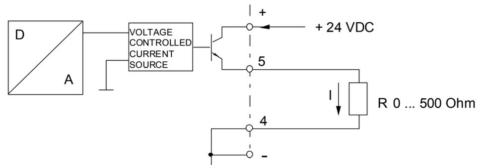
An external 24 VDC supply voltage is required for current outputs.
