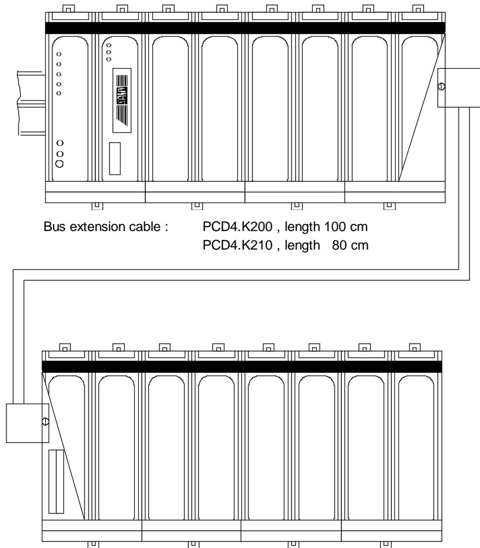
If there is insufficient space for all I/O modules in one row, they can be arranged in a second row above or below the row which contains the processor module.
