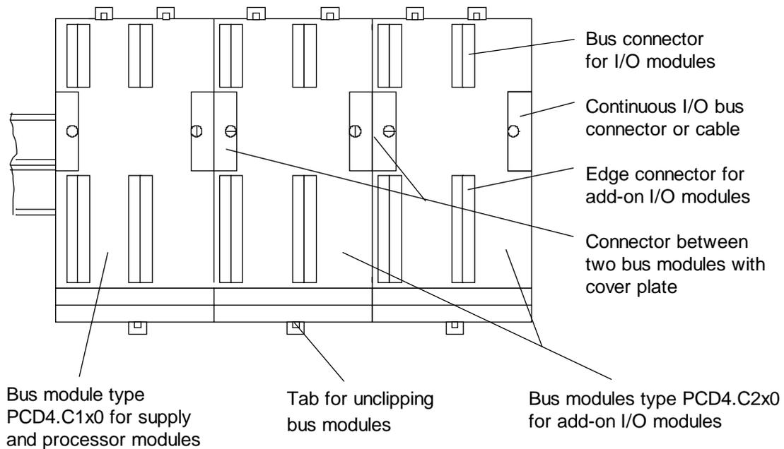
The bus modules for the supply and processor modules must each be installed on the left side of every assembled PCD4 (PCD4.C1x0 or ..C340). The I/O bus modules (PCD4.C2x0) are placed on the right.
