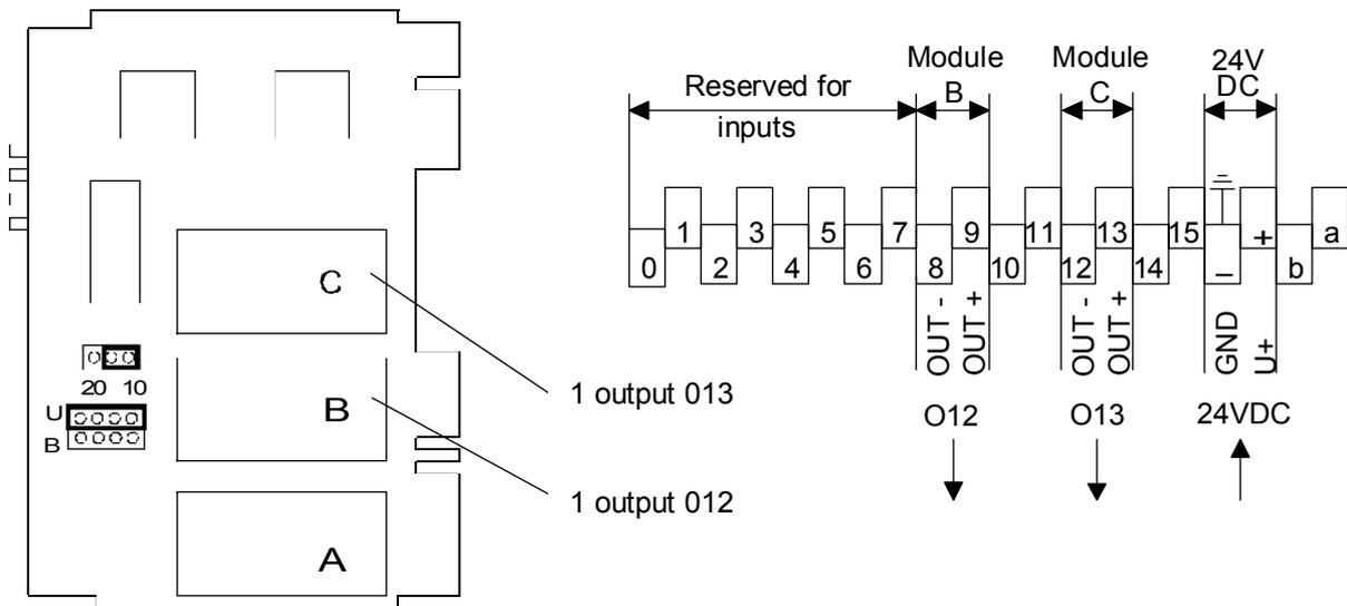
Installing at space B and/or C
