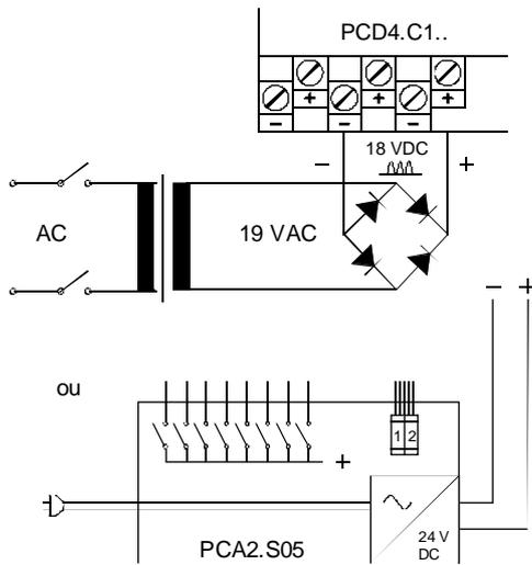
5) Connect 24 VDC smoothed or 18 VDC full wave rectified to terminals + and -. For small-scale requirements, 24 VDC at 0.5 A is adequate. An easy way to do this is to use the PCA2.S05 input simulator (no longer available), which not only provides 16 input switches but also offers 24 VDC.
