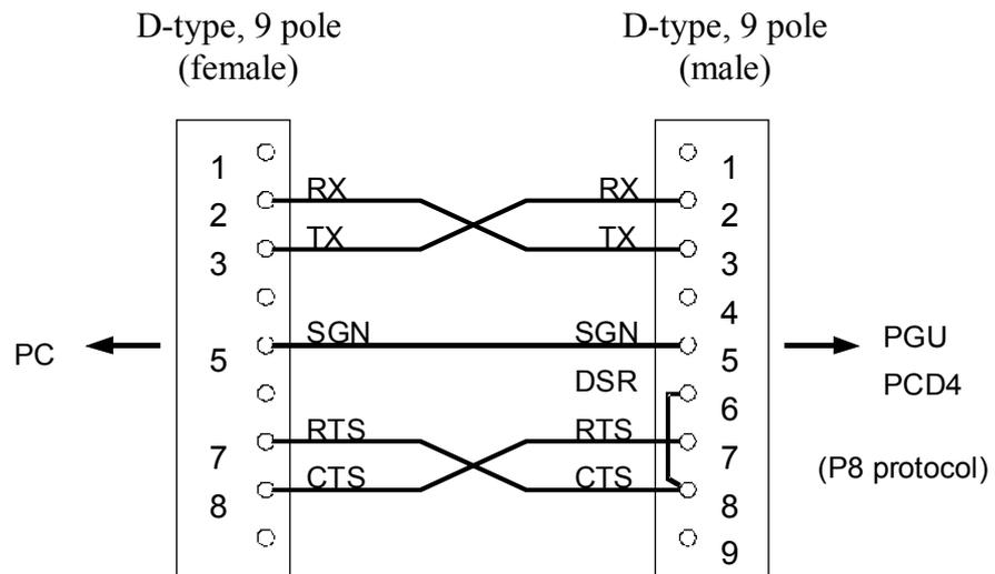
**PCD8.K111 connecting cable** (for P8 and S-Bus protocol)
