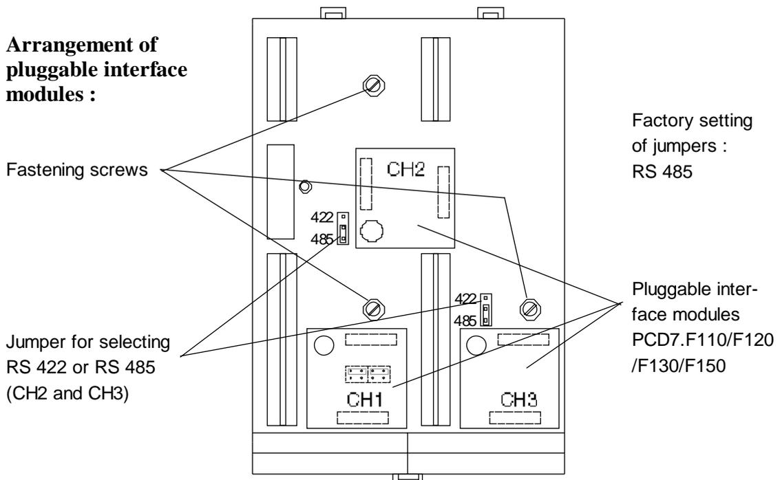
The interface modules can be reached by removing the plastic cover of sockets 1 and 2 (far left cover), which is fastened with 3 screws. The interface modules are now accessible and can be manipulated. After completion of assembly, the cover should be screwed down again.
