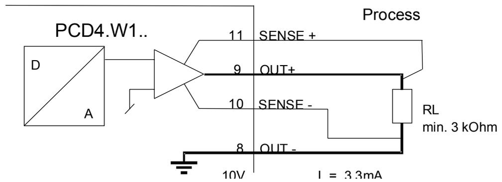
**Note :** Two "SENSE" measurement cables are provided to increase voltage precision at the load resistance  $R_L$ .
