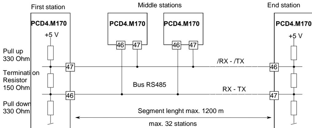
**Note:** It is recommended that the line termination resistors should be included in the cable connector. There are no termination resistors on the module itself.
