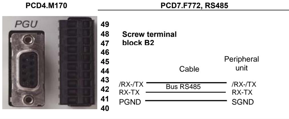
**Selection and connection of line termination resistors**
