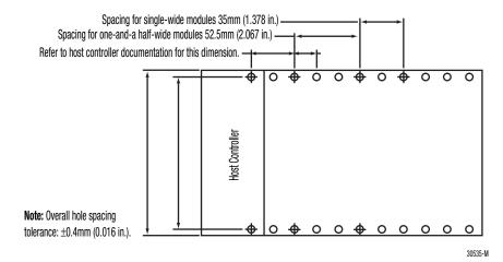
Locate holes every 17.5 mm (0.689 in.) to allow for a mix of single-wide and one-and-a-half-wide modules (e.g., 1769-OA16).
