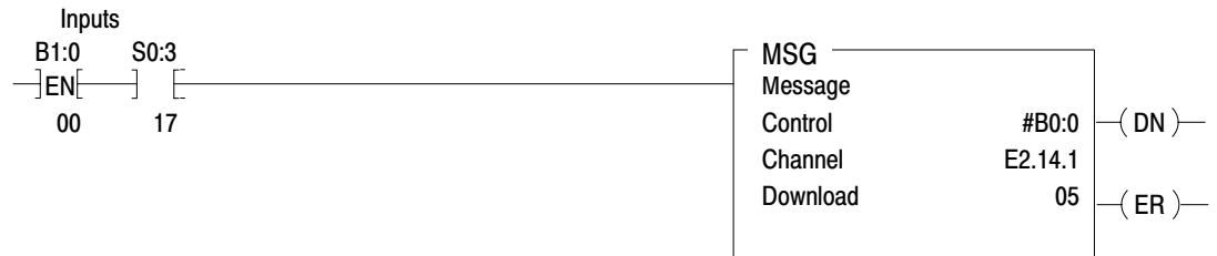
Figure 3.1 Example Rung for Performing Memory Download at Startup
